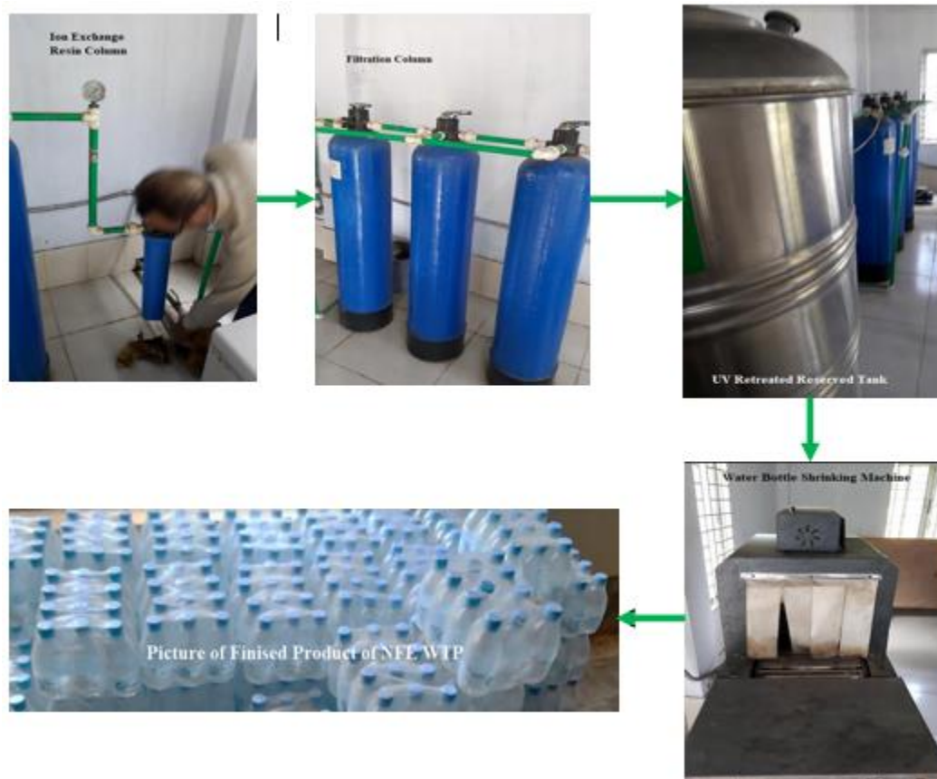
Fig: Water Treatment Plant to use the water for drinking in campus
